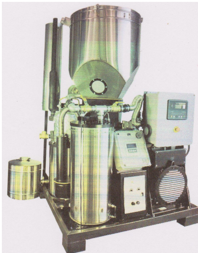
Figure 3- A self-contained Biomass Generator (20 KW)
